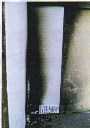
Fig.6 After SBI Test(short wing)
