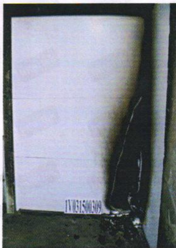
Fig.5 After SBI Test (long wing)
